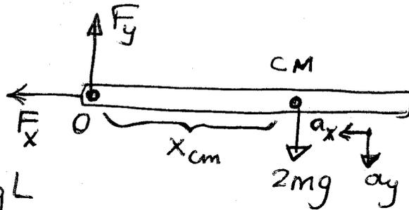
d) We first find angular velocity  $\omega$  by using the conservation of energy
