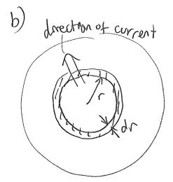
Consider resistors shaped as cylinderical shells as shown  $dR = S \frac{dr}{2\pi r \cdot L} \Rightarrow \frac{S}{2\pi L} \int_{c_{a}}^{b} \frac{dr}{r} = \int_{c_{a}}^{b} dr$
