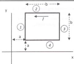
Q5 (5pt). A square loop of wire is placed in the x-y plane as shown in the figure. Side 1 and side 3 are parallel to y-axis, side 2 and side 4 are parallel to x-axis. The loop carries a current I. A magnetic field  $\vec{B} = Cx\hat{i} - Cz\hat{k}$  is applied. Find the force acting on each side of the loop (side 1, side 2, side 3, and side 4).
