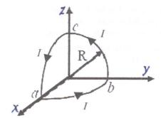
**Q6** (5pt). A wire is bent into three circular segments, each has a radius R. Each segment is a quadrant of a circle, **ab** lying in the **x-y** plane, **bc** lying in the **y-z** plane, and **ca** lying in the **z-x** plane. The wire carries a current I. Calculate the net magnetic field vector  $\vec{B}$  at the origin.
